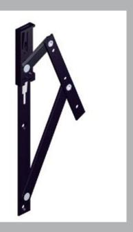
A unique two phase range of 4-bar friction hinges (stays) providing a double operating action for projected top hung (PTH) windows. The first phase allows ventilation whereas the second phase allows the sash to slide into the near horizontal cleaning position. The DA32 double action range is designed to cater for sash weights associated with residential usage up to 18kg.
