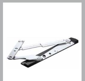
A premier range of 4-bar friction hinges (stays) used for the support and frictional control of projecting side hung (PSH) aluminium, timber or uPVC sashes. Manufactured from 304 grade austenitic (non-magnetic) stainless steel, the range caters for the sizes and weights of sashes normally associated with residential or light commercial applications.
